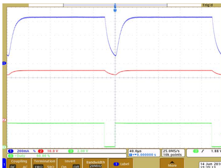
Figure 19. LED Current, LED Voltage, and PDIM Input Waveforms at 90% Duty Cycle
