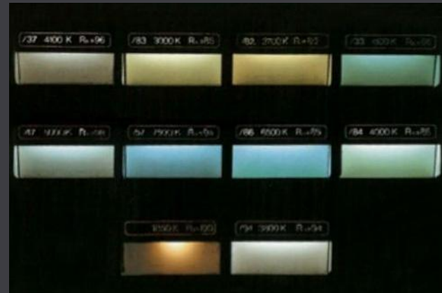
Fig. 6.13. Different TL fluorescent tubes seen together show distinct colors, different from white.
