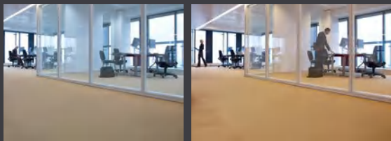
Fig. 5.12. Left: Luminance contrast: cool white correlated color temperature. Right: Luminance contrast: warm white correlated color temperature.
