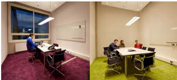
Fig. 8.3. Careful matching of surface reflectances to achieve good and comfortable luminance ratios.
