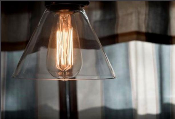
Fig. 6.12. An incandescent lamp in full daylight looks yellowish instead of white.
