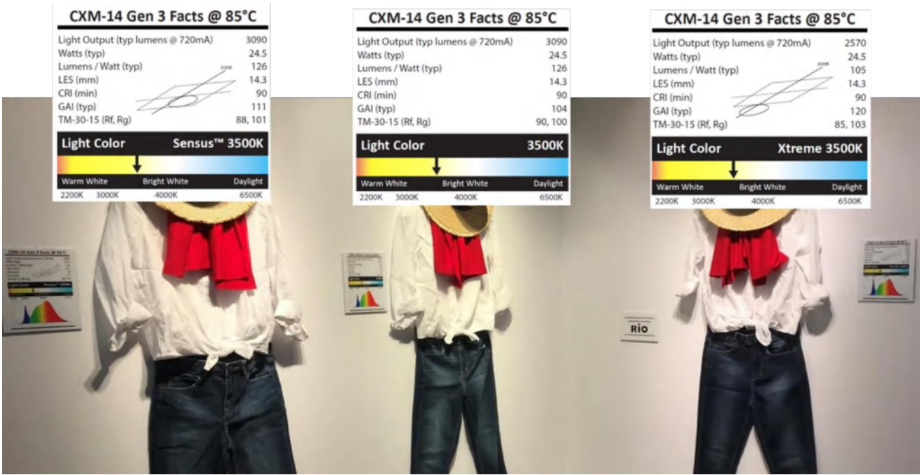
Figure 11 - Three LED bulbs with the same CCT (3500K) and an identical CRI (90) nevertheless render colors differently. The white shirt and the red scarf on the right and left appear visibly brighter; the shirt in the middle has a slightly yellow cast and the red scarf is a cooler tone (less orange, more blue).
