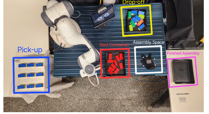
Fig. 4. Top view of the experiment setup. The robot picks up blocks from the “Pick-up” area and puts them in the “Drop-off” area. The participant has to pick blocks from the “Red Container” and “Drop-off” areas, assemble them in the “Assembly Space” area, place the finished assembly in the “Finished Assembly” area, tick the box on the sheet next to that area, and write the color of the assembled top block on the sheet.
